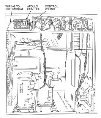
Fig. 5 — Apollo Control Factory-Installed In Typical Unit
